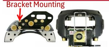
\*Note position of Bracket Mounting\* Left side for LH Caliper Right side for RH Caliper If the I.D tag is still intact you will find the "caliper model" and "part number" located here.
